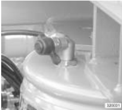
Test connection on pneumatic suspension bellows
